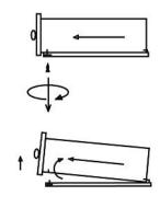
Pull the drawer out until it stops. From underneath the rails, loosen and remove the mounting screws.
